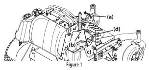
**IMPORTANT:** The mower is equipped with two hydrostatic transmissions. Each transmission is equipped with a bypass valve that MUST be opened before manually moving the mower.
